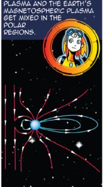
SO AT CERTAIN TIMES SOME OF THE EARTH'S MAGNETIC FIELD LINES IN THE HIGHEST LATITUDE POLAR REGIONS WILL BE CONNECTED DIRECTLY TO THE SOLAR WIND'S MAGNETIC FIELD LINES. WE CALL THESE "OPEN FIELD LINES" BECAUSE ONLY ONE END OF THEM IS CONNECTED TO THE EARTH. SOLAR WIND PLASMA ON THESE LINES CAN GET INTO THE MAGNETOSPHERE AND MAGNETOSPHERIC PLASMA CAN LEAK OUT INTO THE SOLAR WIND. ANY FIELD LINE WITH ITS
