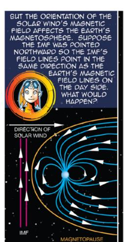
IN THAT CASE IT'S LIKE WHAT HAPPENS IF YOU TRY TO PUSH TWO BAR MAGNETS TOGETHER WHEN THE POLES ARE POINTED THE SAME DIRECTION. THE LINES CAN'T CROSS EACH OTHER AND THE MAGNETS RESIST EACH OTHER.
